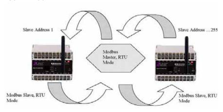
This typical application shows two Slave Modbus controllers. Modbus slave controller can be address from 1 to 255.
